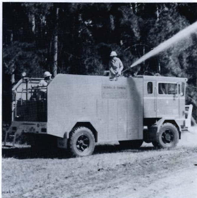
Pictured above the R.F.W. demonstrates the power of spray from the R.F.W. fire hoses and front bumper-wheel sprays.
